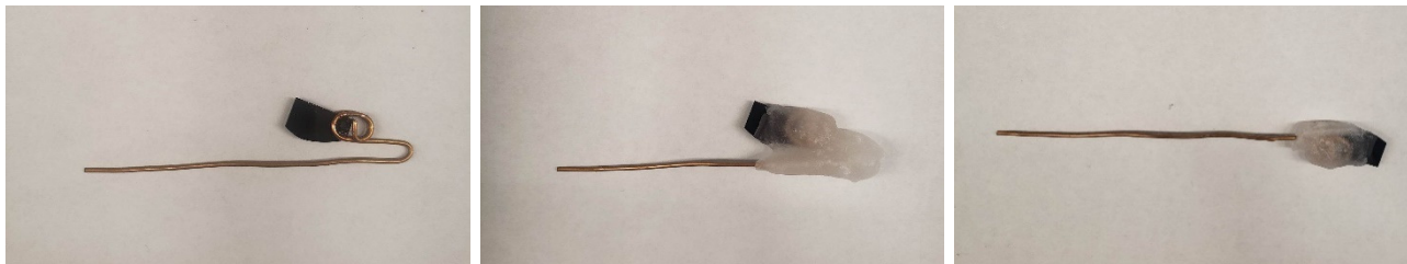
Supplementary Figure 15: Images of electrode preparation steps. Left: Functionalized glassy carbon electrode placed in the loop of a Cu wire and bonded with conductive paste. Middle: Electrode assembly after dipping in wax to seal Cu off from electrolyte. Cu wire was dipped into wax loop first to ensure Cu was sealed without wax contacting exposed glassy carbon. Right: Excess wax is removed and wire is straightened to complete electrode preparation. At no point during electrochemical analysis did the electrolyte rise above the insulating wax layer.
