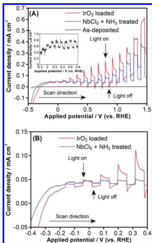
**Figure 1.** (A) Current–voltage curves in aqueous 0.1 M  $\text{Na}_2\text{SO}_4$  solution ( $\text{pH} \approx 6$ ) under intermittent visible-light irradiation ( $\lambda > 420$  nm) for modified  $\text{SrNbO}_2\text{N}$  electrodes ( $2.5 \text{ cm}^2$ ). Scan rate:  $20 \text{ mV s}^{-1}$ . (B) Enlarged view of the lower-potential regions in (A).
