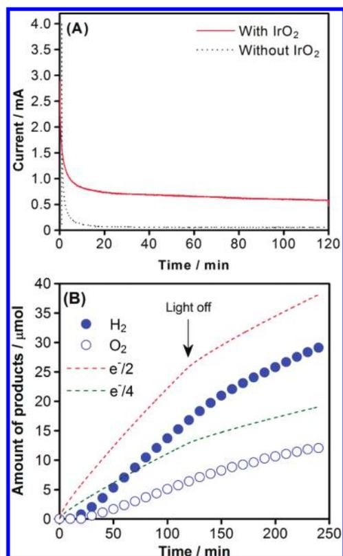
**Figure 2.** (A) Current–time curves in aqueous 0.5 M Na<sub>2</sub>SO<sub>4</sub> solution (pH ≈ 6) for postnecked SrNbO<sub>2</sub>N electrodes (6 cm<sup>2</sup>) with and without modification by colloidal IrO<sub>2</sub> at +1.55 V vs RHE under visible-light irradiation ( $\lambda > 420$  nm). (B) Corresponding time courses of gas evolution in photoelectrochemical water splitting using an IrO<sub>2</sub>-modified electrode.
