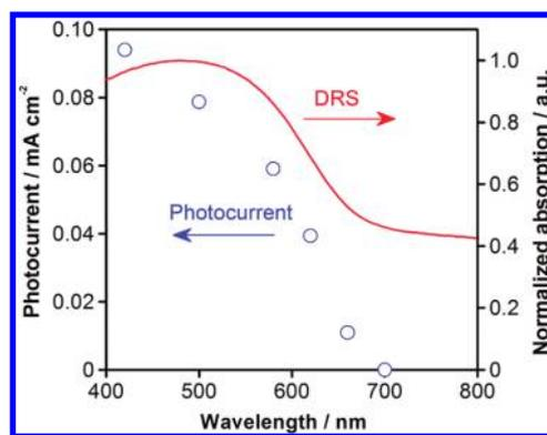
**Figure 3.** Dependence of the photocurrent generated by the IrO<sub>2</sub>-modified SrNbO<sub>2</sub>N electrode (6 cm<sup>2</sup>) at 0.95 V vs RHE in aqueous 0.1 M Na<sub>2</sub>O<sub>4</sub> solution upon the cutoff wavelength of the incident light. The DRS spectrum of SrNbO<sub>2</sub>N is also shown. The spectral features of the light sources are displayed in Figure S14.
