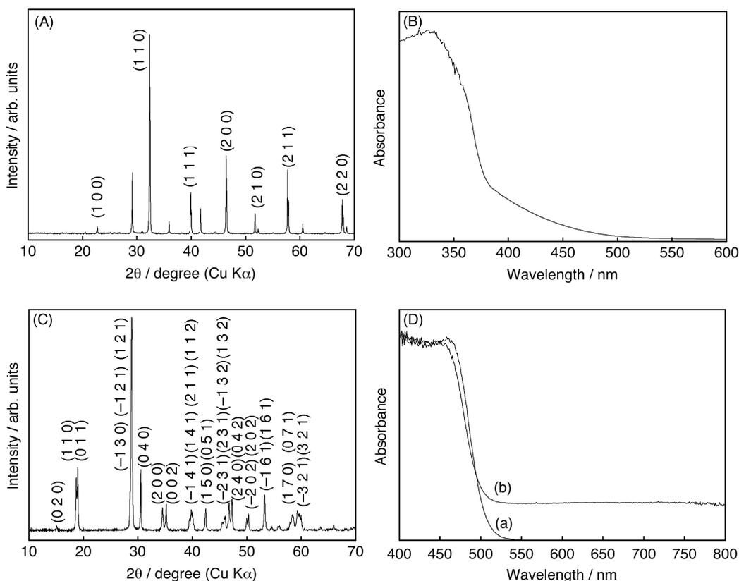
**Figure S1.** XRD patterns of (A)  $\text{SrTiO}_3\text{:Rh}$  and (C)  $\text{BiVO}_4$ , and diffuse reflectance spectra of (B)  $\text{SrTiO}_3\text{:Rh}$  with  $\text{H}_2$ -reduction and (D)-(a)  $\text{BiVO}_4$  and (b) photoreduced graphene oxide/ $\text{BiVO}_4$ .
