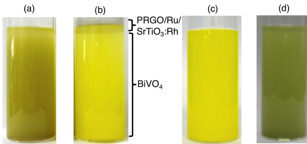
**Figure S2.** Photograph of (a) Ru/SrTiO<sub>3</sub>:Rh and BiVO<sub>4</sub> and (b) photoreduced graphene oxide (PRGO)/Ru/SrTiO<sub>3</sub>:Rh and BiVO<sub>4</sub>, (c) BiVO<sub>4</sub>, and (d) Ru/SrTiO<sub>3</sub>:Rh and PRGO/BiVO<sub>4</sub> suspended in water at pH 3.5.
