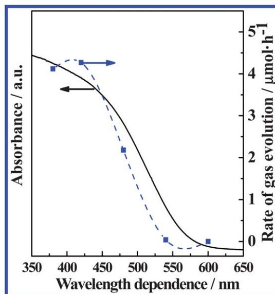
**Fig. 6** Dependence of the  $H_2$  evolution rate on the cutoff wavelength of incident light (dotted line) and the UV-Vis DRS of  $Sr_5Ta_4O_{15-x}N_x$  (solid line). Experimental conditions: 0.3 wt% Pt/ $Sr_5Ta_4O_{15-x}N_x$  (0.15 g);  $La_2O_3$  (0.15 g); 150 mL 20 v% methanol solution system; 1 h irradiation.
