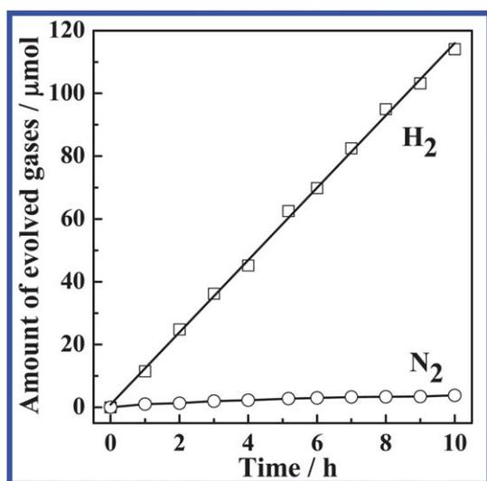
**Fig. 5** Typical time course of photocatalytic  $H_2$  evolution on 0.3 wt% Pt/ $Sr_5Ta_4O_{15-x}N_x$  under visible light irradiation. Reaction conditions: 20 v% methanol solution (150 mL) with 0.15 g catalyst and 0.15 g  $La_2O_3$ ; 300 W Xe lamp ( $\lambda \geq 420$  nm).
