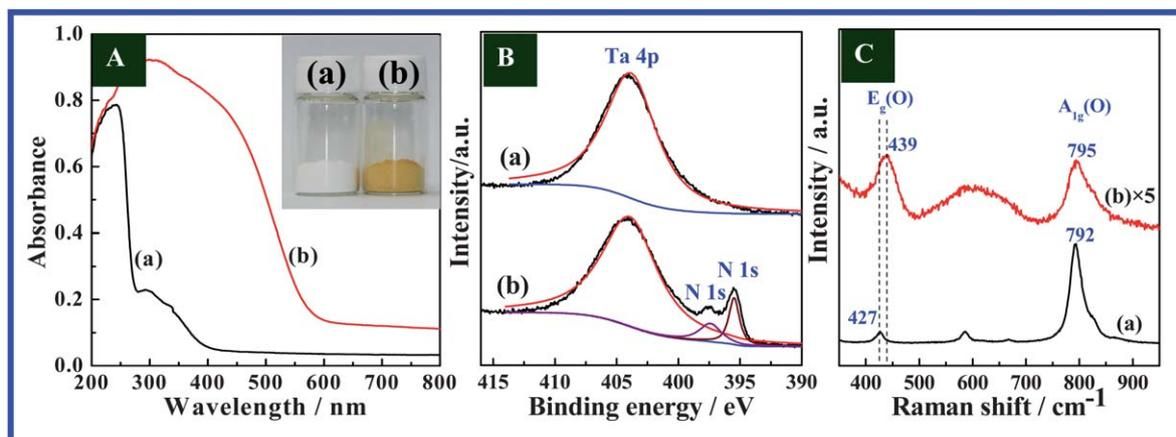
**Fig. 2** Spectral characterizations of  $\text{Sr}_5\text{Ta}_4\text{O}_{15}$  (a) and  $\text{Sr}_5\text{Ta}_4\text{O}_{15-x}\text{N}_x$  (b): (A) UV-Vis DRS (inset shows the photos of samples before and after nitridation); (B) XPS spectra; (C) UV Raman spectra.
