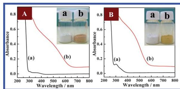
**Fig. 8** UV-Vis DRS and photos (inset) of the samples before and after nitridation: (A)  $\text{Ba}_5\text{Ta}_4\text{O}_{15}$  (a) and  $\text{Ba}_5\text{Ta}_4\text{O}_{15-x}\text{N}_x$  (b); (B)  $\text{Sr}_2\text{Ta}_2\text{O}_7$  (a) and  $\text{Sr}_2\text{Ta}_2\text{O}_{7-x}\text{N}_x$  (b).
