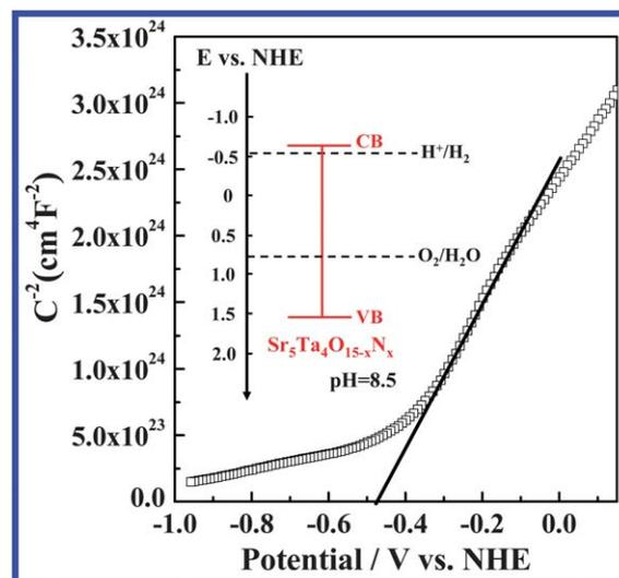
Fig. 4 M–S plot of the Sr<sub>5</sub>Ta<sub>4</sub>O<sub>15-x</sub>N<sub>x</sub> electrode and the estimated band edge positions of Sr<sub>5</sub>Ta<sub>4</sub>O<sub>15-x</sub>N<sub>x</sub> at pH = 8.5 (inset). Electrolyte: 0.1 M Na<sub>2</sub>SO<sub>4</sub> solution (pH = 8.5, adjusted by NaOH); frequency: 3 kHz.
