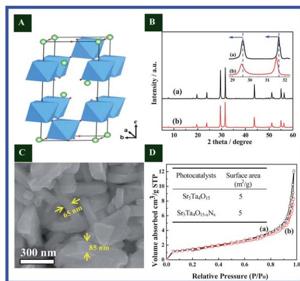
**Fig. 1** Structural characterizations of  $\text{Sr}_5\text{Ta}_4\text{O}_{15}$  (a) and  $\text{Sr}_5\text{Ta}_4\text{O}_{15-x}\text{N}_x$  (b): (A) crystal structure model of  $\text{Sr}_5\text{Ta}_4\text{O}_{15}$ ; (B) XRD patterns; (C) SEM image of  $\text{Sr}_5\text{Ta}_4\text{O}_{15-x}\text{N}_x$ ; (D) adsorption–desorption isotherms.
