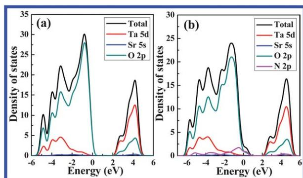
Fig. 3 Density of states of Sr<sub>5</sub>Ta<sub>4</sub>O<sub>15</sub> (a) and Sr<sub>5</sub>Ta<sub>4</sub>O<sub>15-x</sub>N<sub>x</sub> (b).
