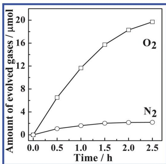
**Fig. 7** Typical time course of  $\text{O}_2$  evolution on the  $\text{CoO}_x/\text{Sr}_5\text{Ta}_4\text{O}_{15-x}\text{N}_x$  under visible light irradiation. Reaction conditions: 0.01 M  $\text{AgNO}_3$  solution (150 mL); 0.15 g catalyst; 0.15 g  $\text{La}_2\text{O}_3$ ; 300 W Xe lamp ( $\lambda \geq 420$  nm).
