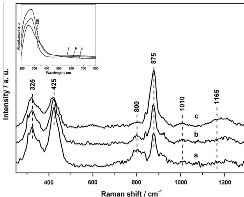
**Fig. 1.** *In situ* UV resonance Raman spectra of the high-temperature-treated Fe/ZSM-35 samples. The excitation laser line: 325 nm. Inset: UV–visible DRS of the high-temperature-treated Fe/ZSM-35 samples. (a) Si/Fe = 320, (b) Si/Fe = 160, and (c) Si/Fe = 80.
