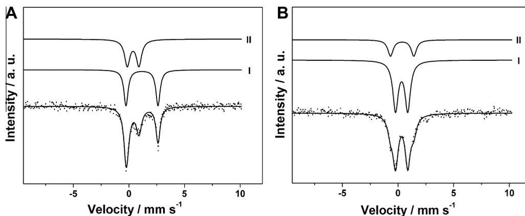
**Fig. 3.** Room temperature  $^{57}\text{Fe}$  Mössbauer spectra of (A) high-temperature-treated Fe/ZSM-35 (Si/Fe = 80) sample and (B) after exposing (A) to  $\text{N}_2\text{O}/\text{He}$  (5.0 vol%) at 523 K.
