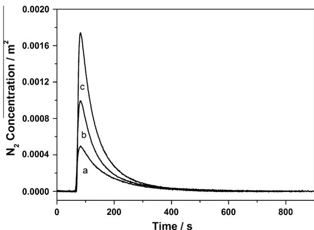
**Fig. 2.** Relationship between the  $\text{N}_2$  concentration normalized by the surface area with different Si/Fe ratios of high-temperature-treated Fe/ZSM-35 samples and the reaction time after a step change from helium to  $\text{N}_2\text{O}/\text{He}$  (5.0 vol%). (a) Si/Fe = 320, (b) Si/Fe = 160, and (c) Si/Fe = 80.
