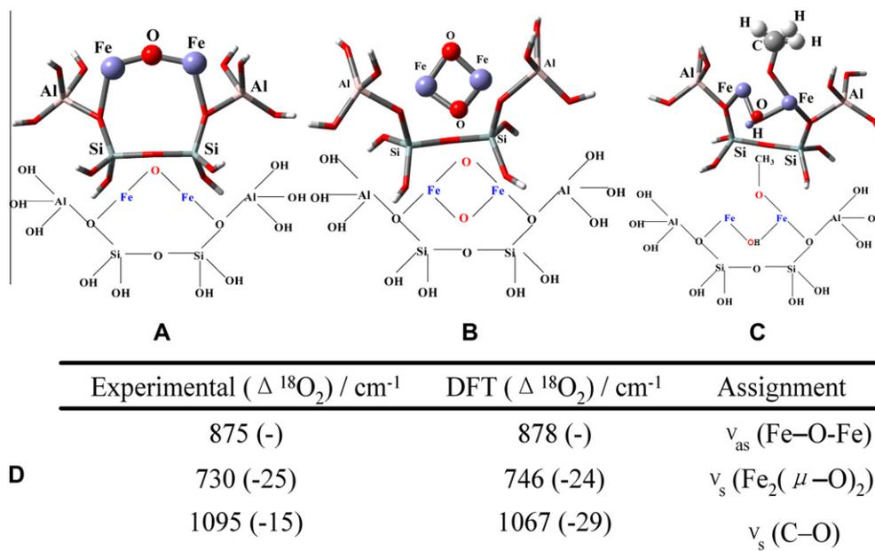
**Fig. 5.** Periodic DFT-optimized structure of (A) the  $\text{Fe}_2(\mu\text{-O})$  site, (B) the  $\text{Fe}_2(\mu\text{-O})_2$  site, and (C) Fe-methoxide species. (D) Comparison of experimentally observed Raman bands with DFT calculated vibrational frequencies ( $^{18}\text{O}$ -isotopic shifts in parentheses) of (A), (B), and (C).
