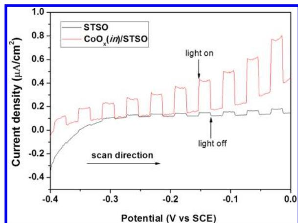
**Figure 4.** Photoanode currents of STSO electrodes with and without cobalt loading in 0.1 M NaOH aqueous solution (pH = 13.0). Scan rate: 10 mV s<sup>-1</sup>.
