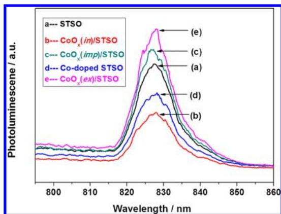
**Figure 5.** Photoluminescence spectra measured at 77 K with 400 nm excitation: (a) STSO; (b) CoO<sub>x</sub>(*in*)/STSO; (c) CoO<sub>x</sub>(*imp*)/STSO; (d) Co-doped STSO; and (e) CoO<sub>x</sub>(*ex*)/STSO.
