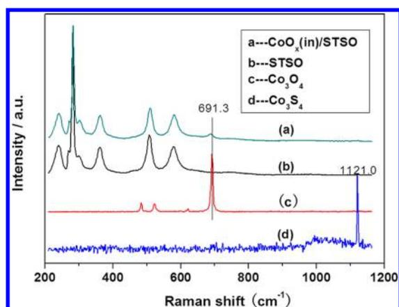
Figure 3. Raman spectra of  $\text{CoO}_x(\text{in})/\text{STSO}$ , STSO,  $\text{Co}_3\text{O}_4$ , and  $\text{Co}_3\text{S}_4$  samples as references.
