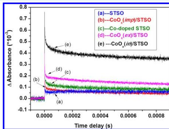
**Figure 6.** Time-resolved infrared absorption (TR-IR) measurements of several typical samples: (a) STSO; (b) CoO<sub>x</sub>(*imp*)/STSO; (c) Co-doped STSO; (d) CoO<sub>x</sub>(*ex*)/STSO; and (e) CoO<sub>x</sub>(*in*)/STSO. The pulse laser at 355 nm (1 Hz, 3 mJ/pulse) was used to excite the samples.
