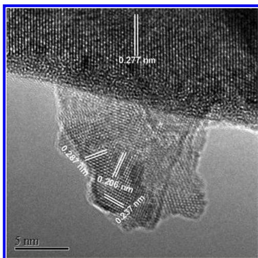
Figure 2. High-resolution TEM image of  $\text{CoO}_x(\text{in})/\text{STSO}$ .
