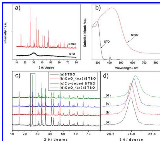
**Figure 1.** Various characterizations of STSO and cobalt-modified STSO samples: (a) XRD patterns; (b) UV–vis spectra; (c, d) XRD patterns of the STSO samples: (a) STSO, (b)  $\text{CoO}_x(\text{ex})/\text{STSO}$ , (c) Co-doped STSO, (d)  $\text{CoO}_x(\text{in})/\text{STSO}$ .
