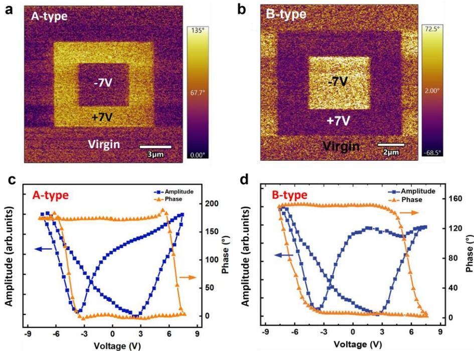
110 **Supplementary Figure S6 | PFM measurement of A- and B-type heterostructures. a, b,**
