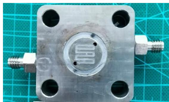
**Supplementary Fig. 39 | Photograph of V2 MEA electrolyzer flow path** with 1 cm<sup>2</sup> active geometric area.
