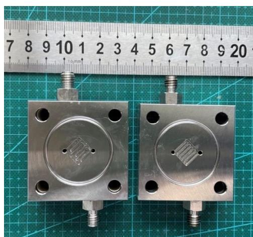
**Supplementary Fig. 36 | Photograph of V1 MEA electrolyzer** with a  $1 \text{ cm}^2$  active geometric area of the flow field on each side.
