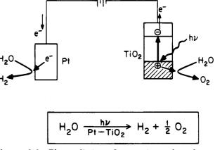
Figure 3.6. Photosplitting of water in a photoelectrochemical cell.
