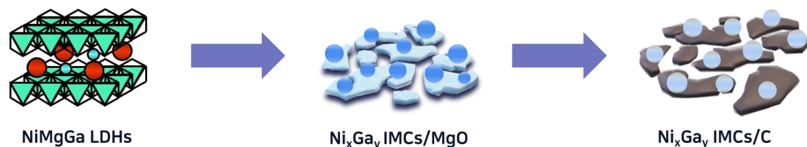
Figure 1. The schematic illustration of synthesizing Nickel Gallium intermetallic compounds derived from layered double hydroxides.
