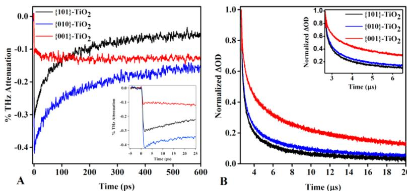
**Figure 5.** (A) Time-resolved THz transients collected from MK-2 sensitized faceted nanoparticle films after photoexcitation with a 400 nm pump beam. (B) Transient absorption curves measured at 800 nm for the decay of the charge-separated state of MK-2 sensitized faceted nanoparticle films after photoinduced electron injection from a pump beam at 560 nm. The insets show the first 25 ps and 7  $\mu\text{s}$  of the TRTS and TA data, respectively.
