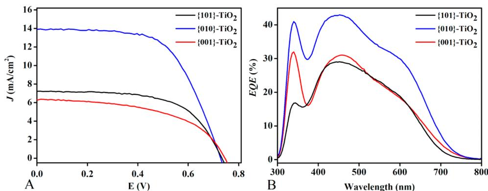
**Figure 3.** Current density vs voltage ( $J$ - $V$ ) under simulated one-sun illumination (A) (AM1.5G) and (B) EQE spectra for DSSC devices prepared with {101}-TiO<sub>2</sub>, {010}-TiO<sub>2</sub>, and {001}-TiO<sub>2</sub>.
