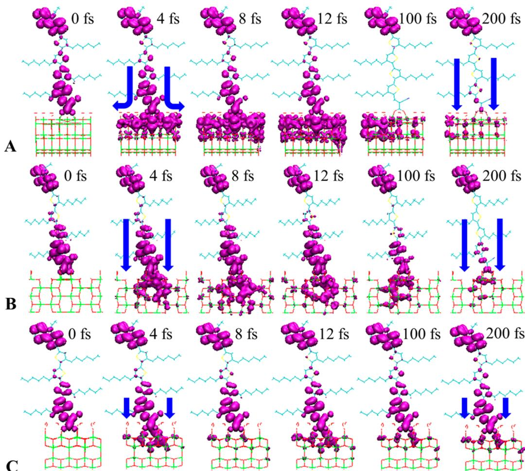
**Figure 7.** Snapshots of electron density calculated at 0, 4, 8, 12, 100, and 200 fs for the (A) {101}, (B) {010}, and (C) {001} facets. The blue arrows denote the direction electron density as it is injected into the TiO<sub>2</sub> facets at the different times.
