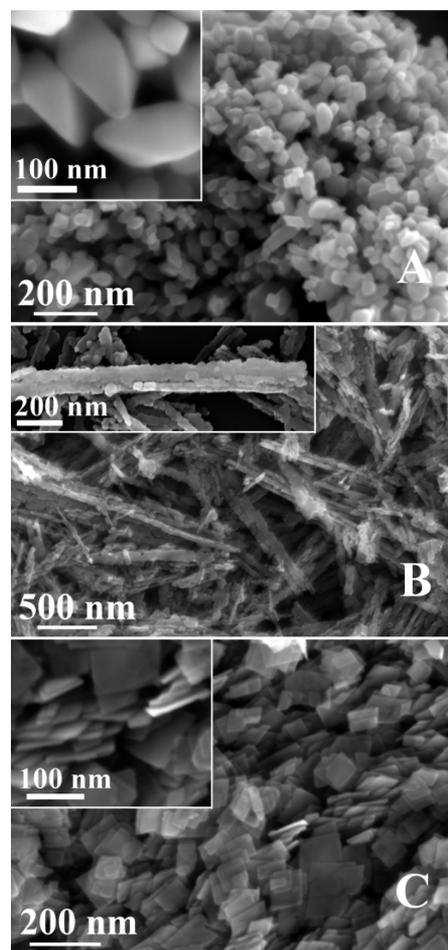
**Figure 1.** SEM images of (A) {101}-TiO<sub>2</sub>, (B) {010}-TiO<sub>2</sub>, and (C) {001}-TiO<sub>2</sub>.
