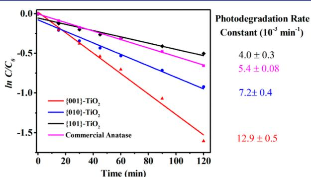
**Figure 2.** Pseudo-first-order plots of the photodegradation of methyl orange using different faceted  $\text{TiO}_2$  and associated photodegradation rate constants.
