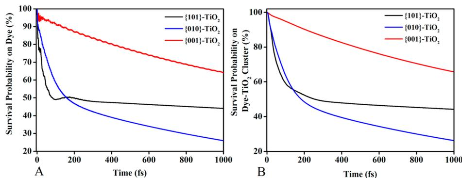
Figure 6. Simulation results for the injection from MK-2 dye bound to the {101}, {010}, and {001} facets via a bridging bidentate interaction. The results are shown as survival probability of electron density on the (A) MK-2 dye and the (B) MK-2 dye and TiO<sub>2</sub> cluster as a function of time.
