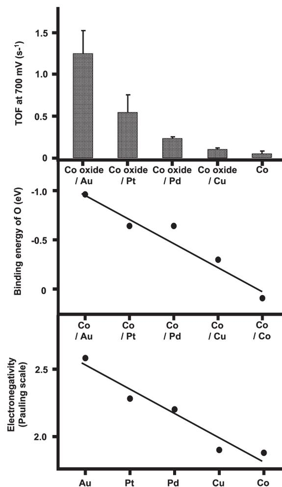
**Figure 5.** A histogram plot of the turnover frequencies of 75  $\mu\text{C}$  cobalt oxide deposited on smooth Au, Pt, Pd, and Cu. The value for Co is also included. The electronegativity of the underlying support as well as the oxygen binding energies of the O–Co/M are also plotted out.
