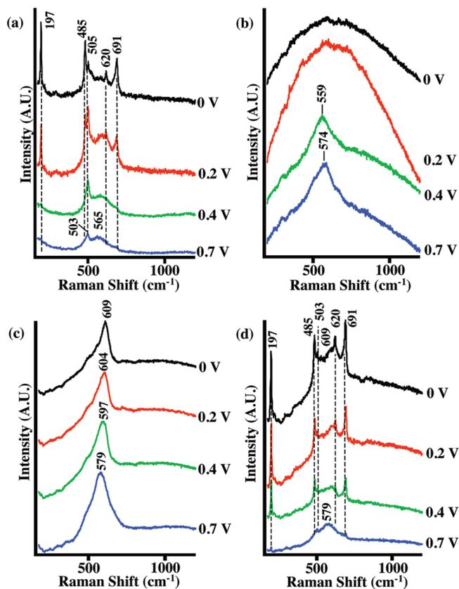
**Figure 3.** In situ Raman spectra of (a) Co surface, (b) Au, (c)  $\sim 0.4 \text{ ML}$  cobalt oxide/Au, and (d)  $\sim 87 \text{ ML}$  cobalt oxide/Au in  $0.1 \text{ M KOH}$ . All the spectra were collected in real time during linear sweep voltammetry scans at  $2 \text{ mV s}^{-1}$ . The acquisition times for the surface-enhanced and normal Raman spectra are 5–6 and 15 s, respectively.
