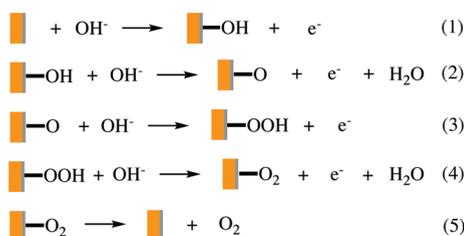
**Figure 6.** A schematic diagram depicting the mechanism for electrochemical oxygen evolution reaction on cobalt oxide/Au. The cobalt oxide (gray) overlayer is above the Au support (gold).
