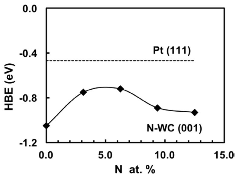
**Supplementary Figure 1 | Correlation of hydrogen binding energy (HBE) with different N doping amount on N-WC (001).** The 6.25 % N doping amount shows the most appropriate HBEs in N-WC.
