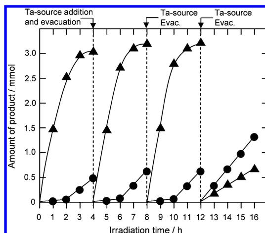
**Figure 7.** Time courses of gas evolution during photodeposition of  $\text{Ta}_2\text{O}_5$  (5 + 5 + 5 wt %) and subsequent water splitting reactions on  $\text{Rh}_2\text{O}_3$  (0.5 wt %)/ $\text{SrTiO}_3\text{:Sc}$ . Catalyst, 0.1 g; solution,  $\text{H}_2\text{O}$  (250 mL); light source, Xe lamp (300 W, full arc). Filled circles,  $\text{H}_2$ ; filled triangles,  $\text{O}_2$ .
