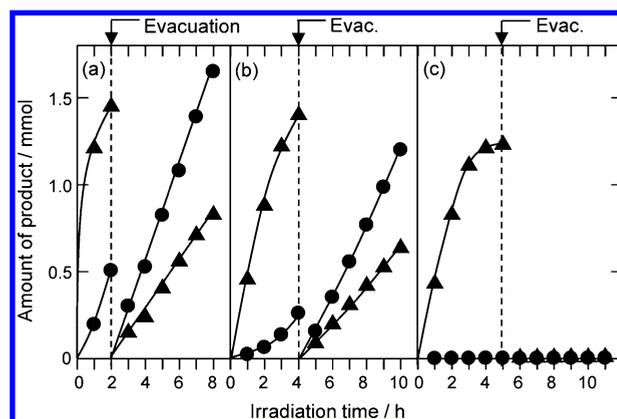
**Figure 3.** Time courses of gas evolution during photodeposition of  $\text{Ta}_2\text{O}_5$  (2 wt %) and the subsequent water splitting reactions on variously modified  $\text{SrTiO}_3:\text{Sc}$ . (a)  $\text{Rh}_2\text{O}_3$  (0.5 wt %)-loaded, (b)  $\text{RhCrO}_x$  (0.5 + 0.5 wt %)-loaded and (c) nonloaded. Catalyst, 0.1 g; solution,  $\text{H}_2\text{O}$  (250 mL); light source, Xe lamp (300 W, full arc). Filled circles,  $\text{H}_2$ ; filled triangles,  $\text{O}_2$ .
