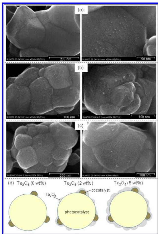
**Figure 4.** SEM micrographs of (a)  $\text{Rh}_2\text{O}_3$  (0.5 wt %)/ $\text{SrTiO}_3\text{:Sc}$ , (b)  $\text{Ta}_2\text{O}_5$  (2 wt %)/ $\text{Rh}_2\text{O}_3$  (0.5 wt %)/ $\text{SrTiO}_3\text{:Sc}$ , and (c)  $\text{Ta}_2\text{O}_5$  (5 wt %)/ $\text{Rh}_2\text{O}_3$  (0.5 wt %)/ $\text{SrTiO}_3\text{:Sc}$ . (d) Schematic of morphological changes.
