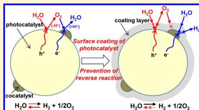
the prevention of the reverse reaction. The photodeposited selectively filtering reactant and product molecules. By exploiting on the photocatalyst surface could be suitably controlled, which
