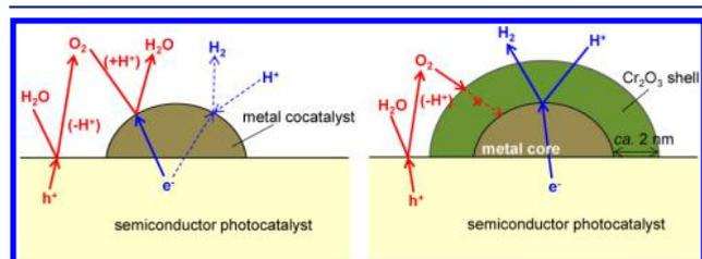
**Figure 1.** Schematic of the function of the core–shell-structured cocatalyst.
